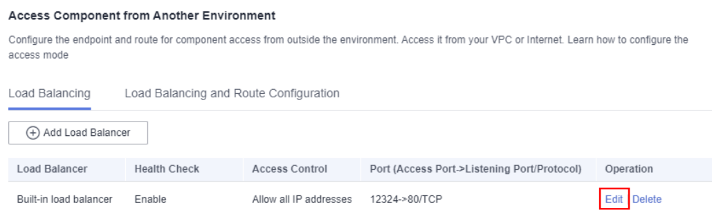
Figure 7-20 Modifying a load balancing configuration
